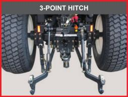
The category 1 hitch has a lift capacity of 1650 kg at the ball end.
