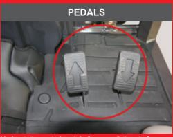
Hydrostatic control pedals for smooth hands free forward and reverse motion.
