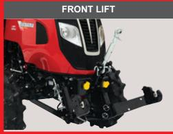
Front lift cat. 1 with a lifting capacity of 1500 kg.
