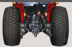
The category II three-point hitch has a lifting capacity of 1500 kg between the balls.
